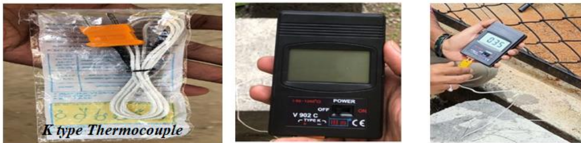
Fig. 6 K type Thermocouple and Temperature Reading Meter
