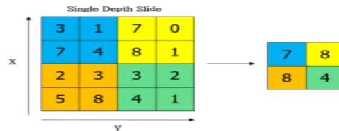
Figure 4: Max Pooling with a 2 \times 2 filter and stride = 2
