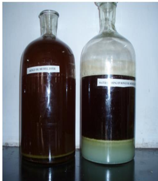
Figure 6: Washing and moisture removal from HOME
