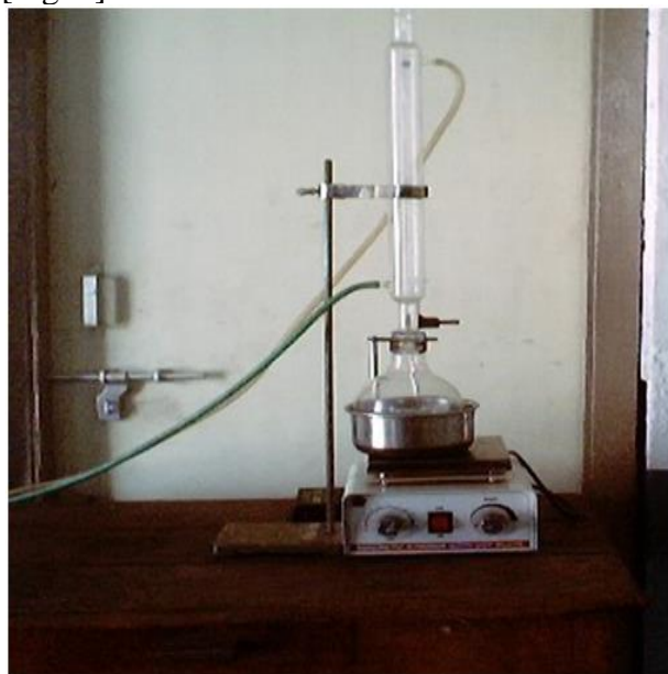
Figure 3: Equipment for Transesterification
