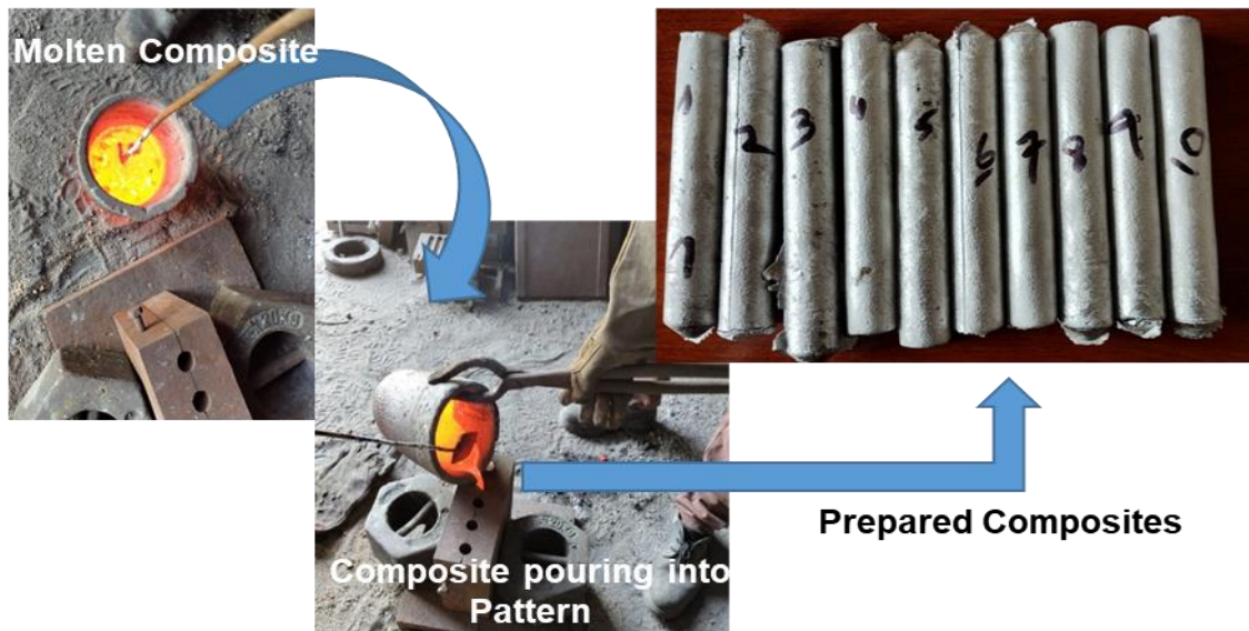
Fig. 1. Al7075/TiC/Gr Composite preparation for tensile testing Table 1: Composition details of Al7075/TiC/Gr hybrid composite samples
