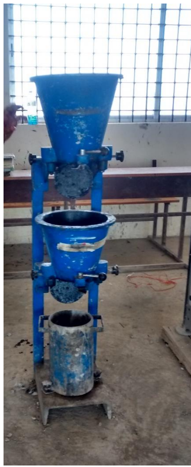
Fig. 13 Compaction factor test
